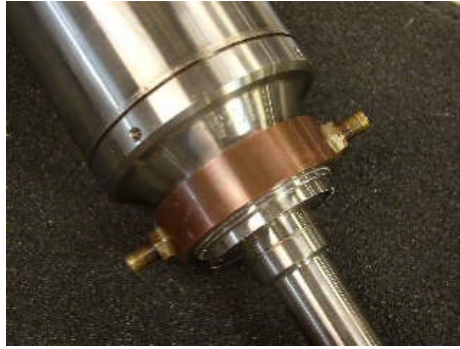
Figure 11: Water Jacket Heat Rejection
